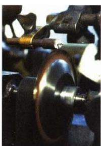
Using a machine to cut a diamond
