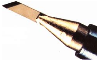
The scalpel has a blade made from metal and diamond dust.
